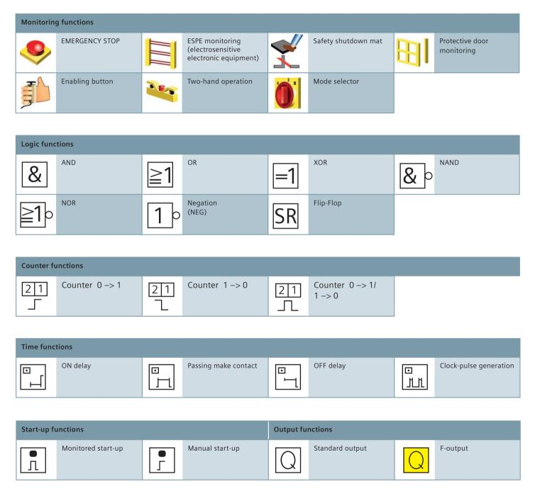
Whatever your safety requirements – all conventional safety functions can be parameterized and operated with the 3RK3 Modular Safety System and the parameterization software. The monitoring functions can be logically interlinked via the logic functions.
